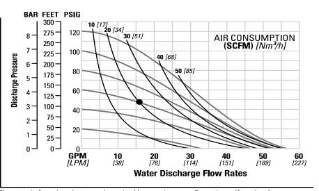
Flow rates indicated on chart were determined by pumping water. For optimum life and performance, pump should be specified so that daily operation parameters will fall in the center of the pump's performance curv
