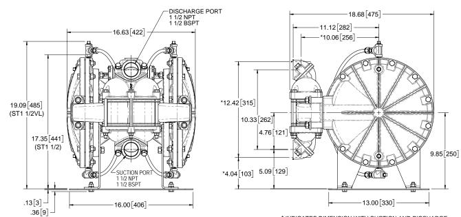
$^{\star}$  INDICATES DIMENSION WITH SUCTION AND DISCHARGE PORTS ROTATED 180  $^{\circ}$  TO A VERTICAL POSITION
