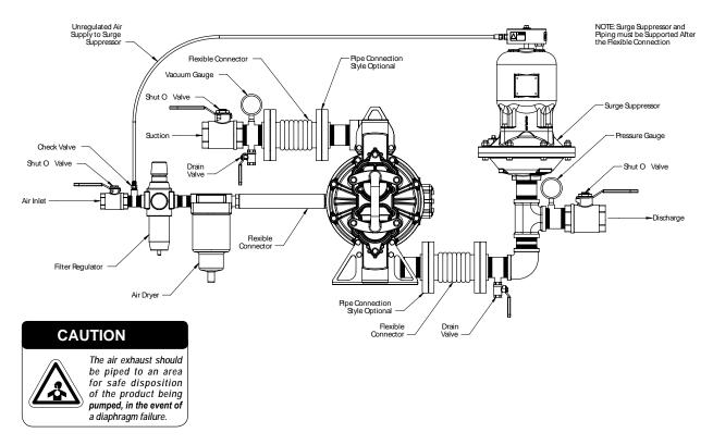
Locate the pump as close to the product being pumped as possible. Keep the suction line length and number of fittings to a minimum. Do not reduce the suction line diameter.
