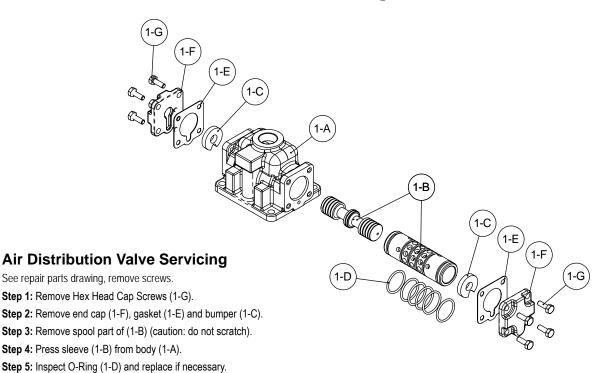
**Step 6:** Lightly lubricate O-Rings (1-D) on sleeve (1-B). **Step 7:** Press sleeve (1-B) into body (1-A).
