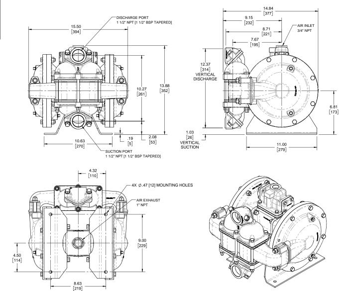
Model HDB1 $\frac{1}{2}$ -A features 1 $\frac{1}{2}$ " NPT threaded connections. Model HDB40-A features 1 $\frac{1}{2}$ " BSP Tapered connections.
