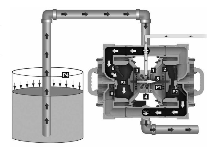
Air-Operated Double Diaphragm (AODD) pumps are powered by compressed air or nitrogen.
