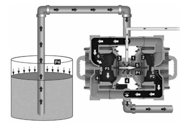
Air-Operated Double Diaphragm (AODD) pumps are powered by compressed air, natural gas or nitrogen.
