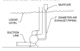
Pump can be submerged if the pump materials of construction are compatible with the liquid being pumped. The gas exhaust must be piped above the liquid level. When the pumped product source is at a higher level than the pump (flooded suction condition), pipe the exhaust higher than the product source to prevent siphoning spills.
