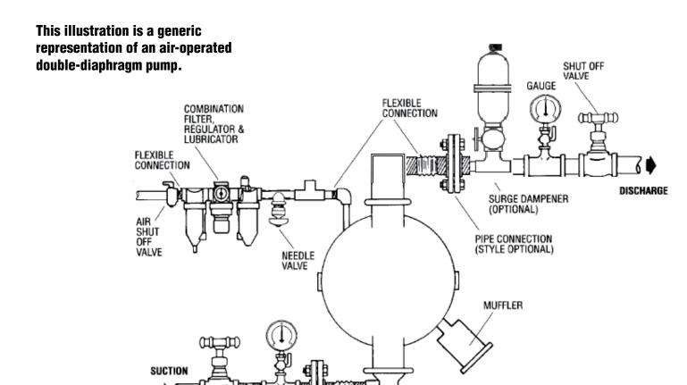
**NOTE:** In the event of a power failure, the shut off valve should be closed, if the restarting of the pump is not desirable once power is regained.
