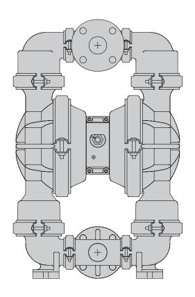
AIR-OPERATED O DOUBLE DIAPHRAGM O PUMPS
