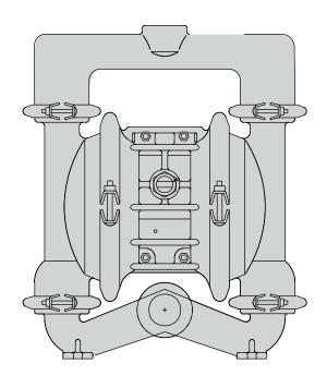
AIR-OPERATED O DOUBLE DIAPHRAGM O PUMPS
