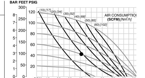
Flow rates indicated on chart were determined by pumping water.
