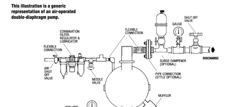
**NOTE:** In the event of a power failure, the shut off valve should be closed, if the restarting of the pump is not desirable once power is regained.
