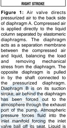
free to move past the inlet valve ball and fill the liquid chamber
