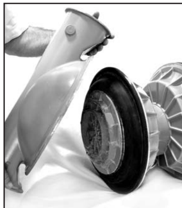
Step 7: Lift liquid chamber away from center section to expose diaphragm and outer piston.
