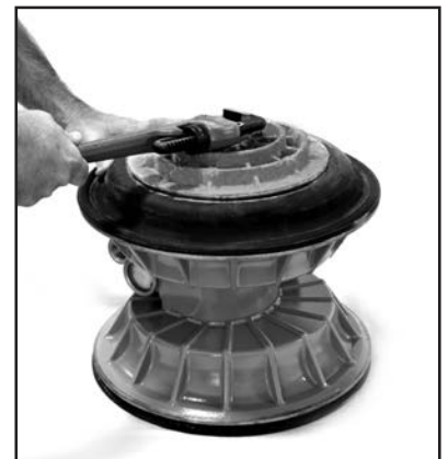
Step 8: Using an adjustable wrench, or by rotating the diaphragm by hand, remove the diaphragm assembly.
