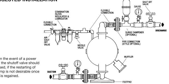
Note: In the event of a power failure, the shutoff valve should be closed, if the restarting of the pump is not desirable once power is regained.
