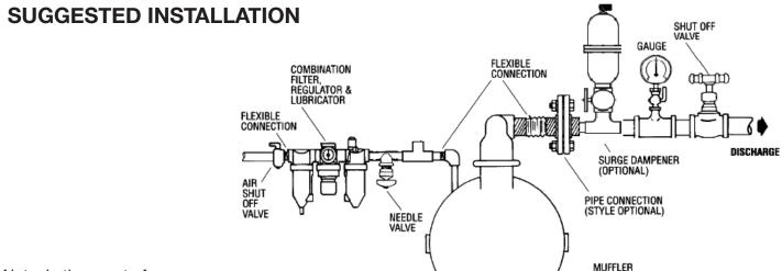
Note: In the event of a power failure, the shutoff valve should be closed, if the restarting of the pump is not desirable once power is regained.
