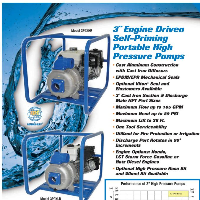
IPT 3" Self-Priming Engine Driven Portable High Pressure pumps are cast aluminum construction with cast iron volute and male NPT ports. Pump applications include fire protection, agricultural spraying, and irrigation. These pumps are available with a wide choice of standard and heavy duty gasoline or diesel fueled engines. These pumps feature closed cast aluminum impeller. All models come equipped with EPDM/EPR elastomers and seals. Most models include a heavy duty steel roll frame.
