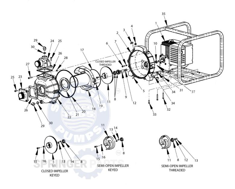
Figure 1 - Repair Parts Illustrations
